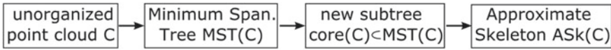
Fig. 2 Pipeline to compute an Approximate Skeleton ASk(C) : MST(C) is classical, the new subtree core(C) \subset MST(C) is introduced in Definition 6 in Sect. 3, final ASk(C) is built in Sect. 4
