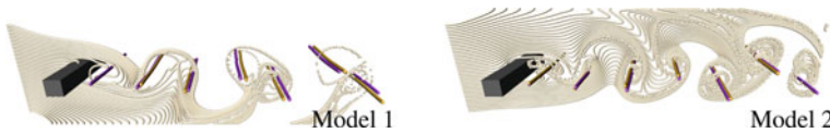
Fig. 5 Comparison of inertial (●) and massless (●) vortex corelines in the flow behind a SQUARE CYLINDER for Model 1 (top, r = 0.25 ) and Model 2 (bottom, R = 0.8 and St = 0.4 ). The heavy aerosol particles of Model 1 are dragged down by gravity \mathbf{g} = (0, -1, 0) while the parameters of Model 2 represent bubbles, which rise upward
