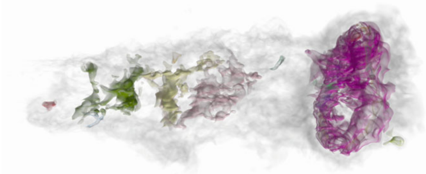
Fig. 1 Distributed topology-controlled volume rendering of the jet data set. Branch pruning minimal persistence is set to 3 (max 16.63)
