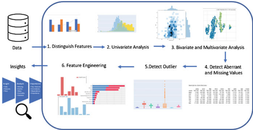
Fig. 2.1 Exploratory data analysis showing various techniques employed to convert data into insights
