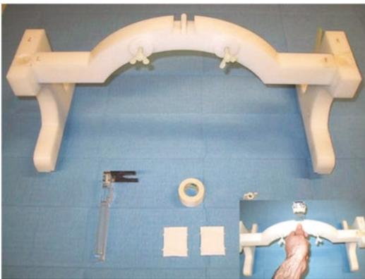
**Fig. 7** A custom build bite-bar system used to minimize patient motion during the fMRI experiment. It consists of a plastic bridge which is positioned over the subject's shoulder and a small detachable piece which the subject puts in his mouth
