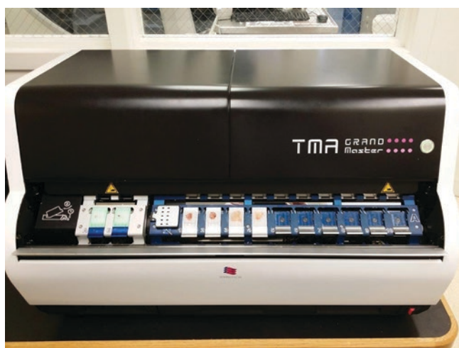
Fig. 11.2 Example of an automated tissue arrayer system (3DHitech; Budapest, Hungary)
