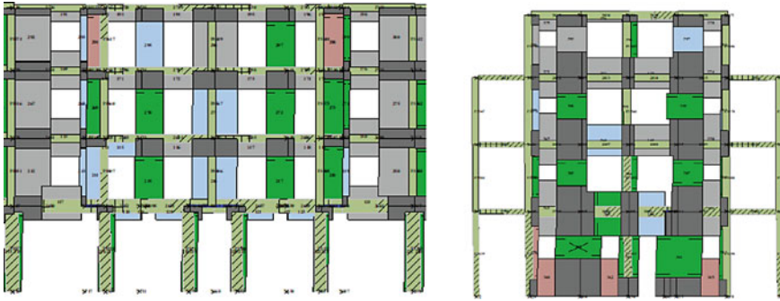
Fig. 11 Damage pattern for C12 (see Fig. 5)
