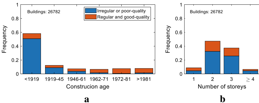
Fig. 5 Subdivision of URM buildings from the completely-surveyed municipalities based on construction age a and number of stories b
