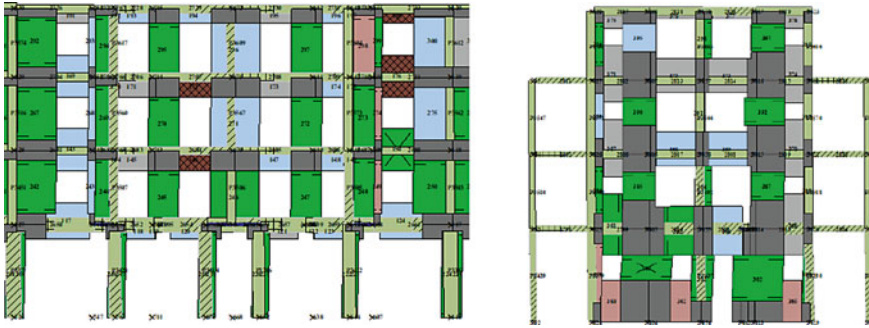
Fig. 9 Damage pattern for C8 (see Fig. 5)
