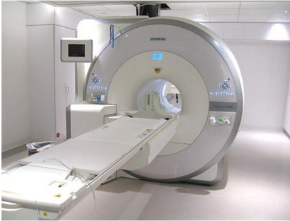
Fig. 13.2 The Siemens biograph hybrid mMR. The white (innermost) circumference represents the PET detectors within the MRI bore (grey bore). (Adjusted and reproduced with permission from Muzic RF, Jr., DiFilippo FP. Positron emission tomography-magnetic resonance imaging: technical review)
