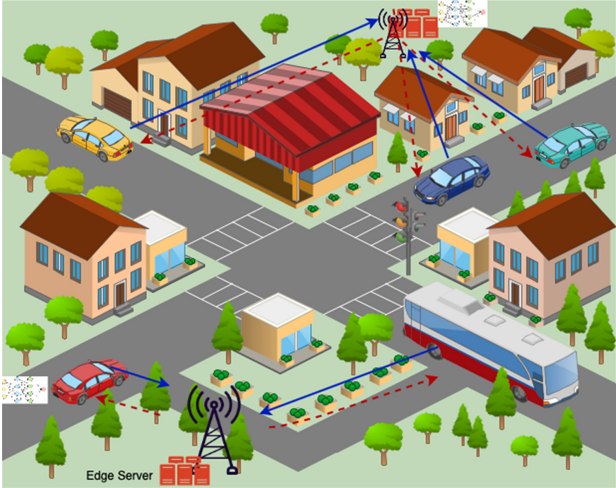
Fig. 1. Communication process of AVs federated learning in edge cloud
