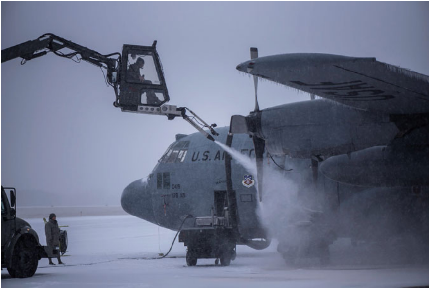
Fig. 8.1 Wing of an airplane with accretions of glaze ice. Title: Ohio National Guard. Author: The National Guard. Source https://flic.kr/p/2iryRE . License: CC BY 2.0. Description: “Airmen work on a C-130H Hercules, spraying it with deicing fluid during a snowstorm, Feb. 07, 2020, at the 179th Airlift Wing, Mansfield, Ohio.”
