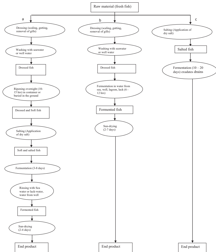
Fig. 17.1 Flow diagram of traditional processing of fermented fish products in Africa. (a) Fermentation with salting and drying, (b) Fermentation and drying without salting (c) Fermentation with salting without drying. (Source: Anihouvi et al. 2012)
