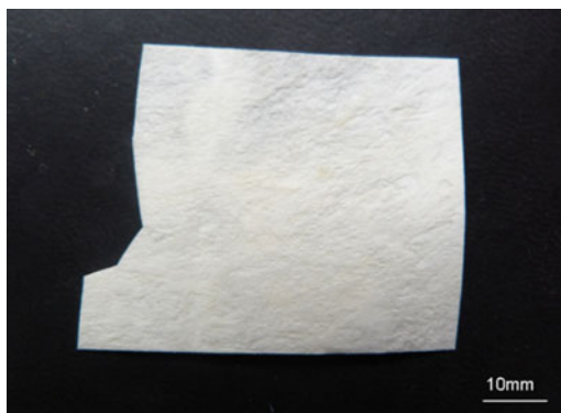
Fig. 10.4 Sheet of one-ply UBM scaffold that was prepared according to the standardised manufacturing protocol. (scale bar represents 10 mm)
