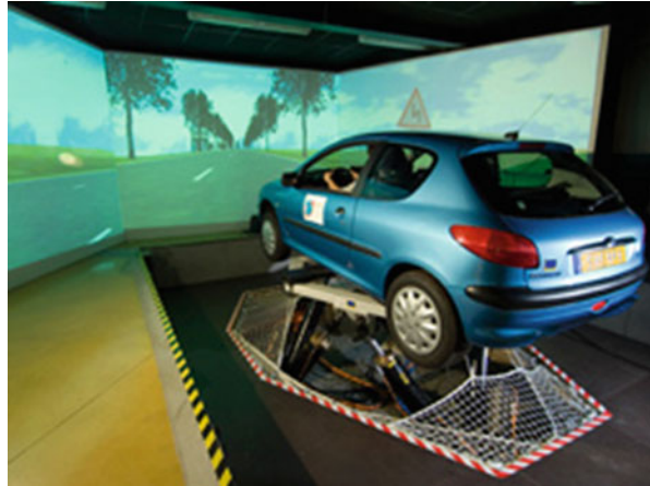
Fig. 8.3 SHERPA simulator used for automotive studies [118]
