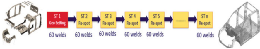
Fig. 7.6 Body Framing diagram of a 45 JPH production line
