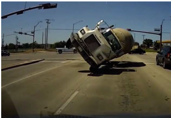
Fig. 13.1 Rollover of a single unit heavy vehicle [8]
