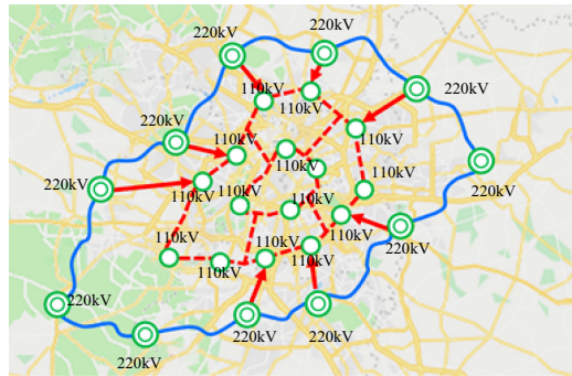
Fig. 2. Regional distribution network structure
