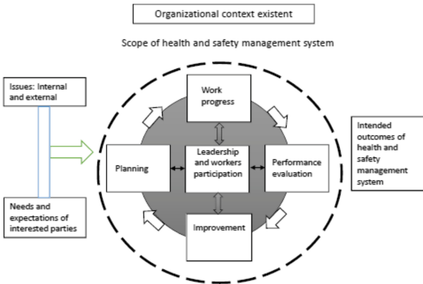
Fig. 1 Flowchart on the concept of management the process of occupational health and safety according to ISO 45001:2018 [4]
