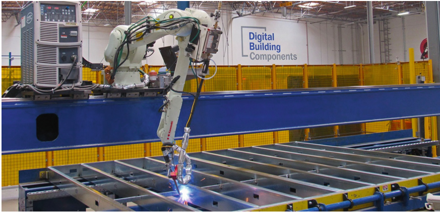
Fig. 8 Automated prefabrication line at Digital Building Components
