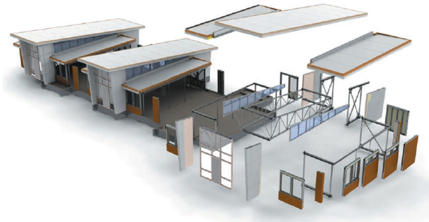
Fig. 7 Example of a kit-of-parts developed by Project Frog
