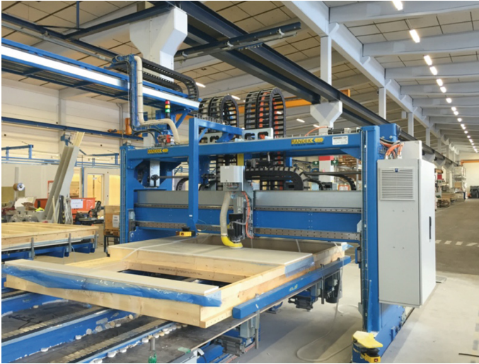
Fig. 4 Automated wall-panel nailing at the BoKlok factory
