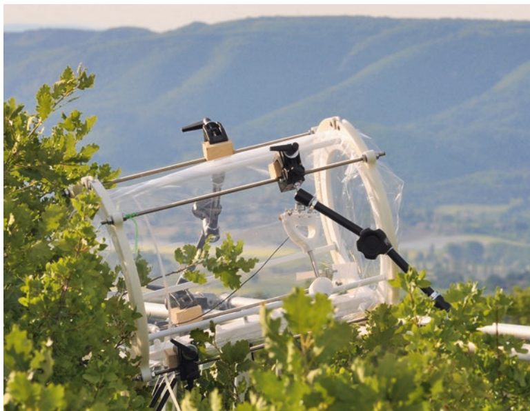
Fig. 1 Dynamic branch enclosure (60 L) system used in the field to study BVOC emissions from Q. pubescens in southern France at O 3 HP deployed during the CANOPEE campaigns (Genard-Zielinski et al., 2015)
