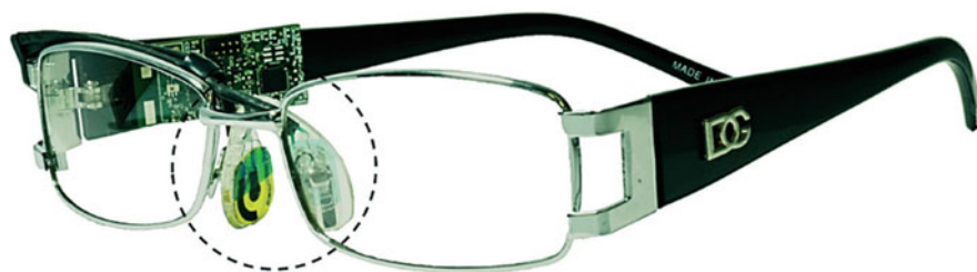
Fig. 4 Real image of the eyeglasses biosensor system integrated with a wireless circuit board along the arms (with permission) (Sempionatto et al. 2017)
