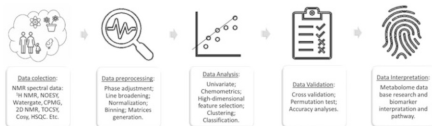
Fig. 2 The accurate metabolomics spectral analyses are divided into five main segments: spectral data collection, data preprocessing—preparations of the matrices, statistical analyses of the spectral data, data validation, and interpretation of the results
