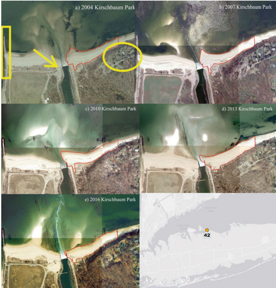
Fig. 33 Northport. Images from Northport, site: Kirschbaum Park. Images (a–e) are 2004, 2007, 2010, 2013, and 2016, respectively. This site is located in a park next to a residential area, indicated by the circle. The arrow points to a manmade canal. The rectangle points out a jetty that keeps open an inlet next to this site
