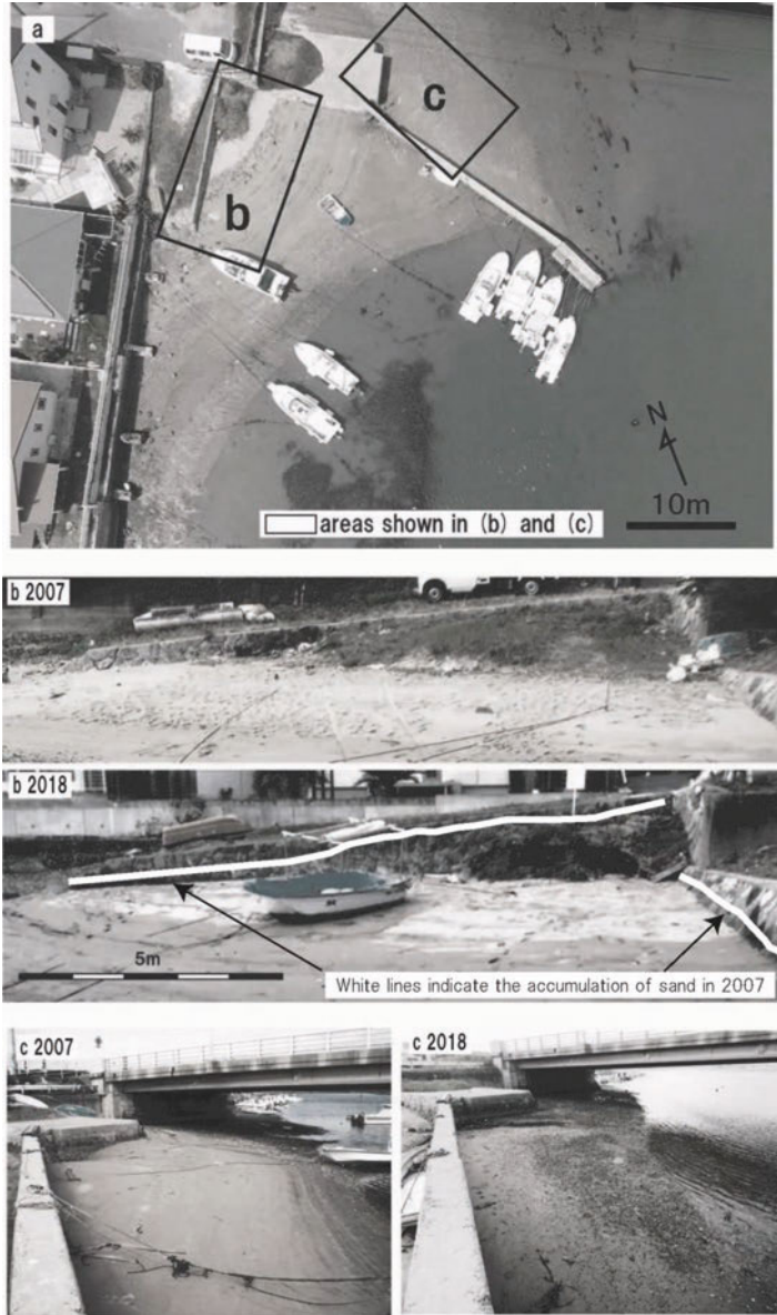
Fig. 8 Comparison of beach morphology and condition at site 2 between 2007 and 2018. (a) Birds-eye view, showing the two studied areas, b and c. (b) Comparison of the sand accumulation at b area in 2007 (above) and in 2018 (below). (c) Comparison of the sand accumulation at c area in 2007 (left) and in 2018 (right). Photos by Shinji Itaya, (a), (b) 2018, (c) 2018, and Masami Sadanaga, (b) 2007, (c) 2007
