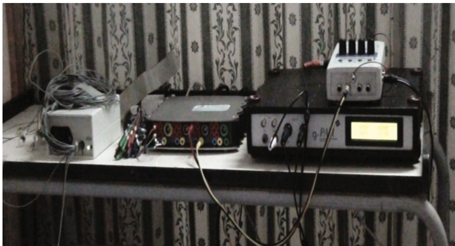
Fig. 1. Hardware system setup with g-tech equipment which include gUSBamp, gPAH, trigger box and Sound Card.
