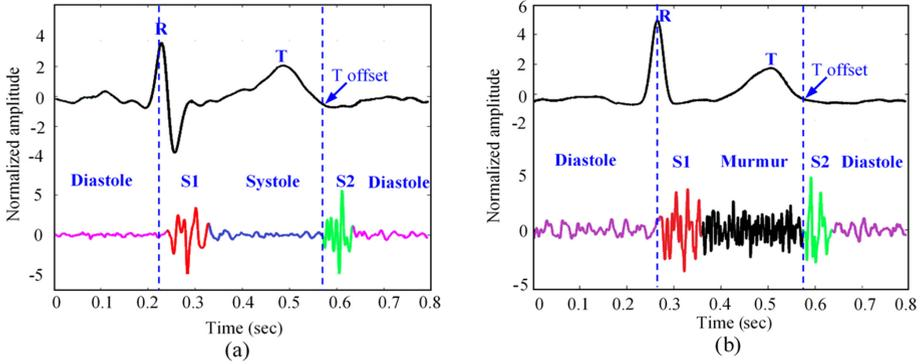
**Fig. 2.** The heart electromechanical activity in the form of ECG and heart sound (PCG) signals. Showing the fundamental heart sound (PCG) components along with the reference ECG graph. (a) Shows an example of normal heartbeat (record a0068 from [9]), (b) shows an example of abnormal heartbeat (record a0002 from [21]).
