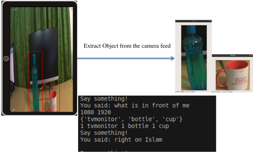
Fig. 7. System performance of ALO for object detection.
