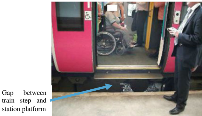
Fig. 1 Horizontal and vertical gaps. Source Emmanuel Matsika, author
