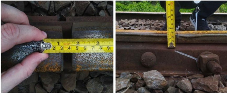
Fig. 8 Top view and side view of the level joint with gap between rails
