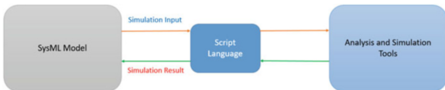
Fig. 1 SysML executable modeling framework
