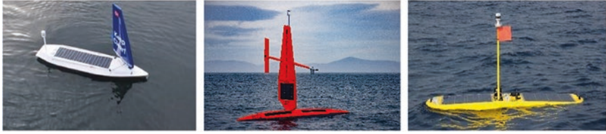
Fig. 3.19 From left to right: a Sailbuoy ( http://www.sailbuoy.no – photo credit David Peddie on behalf of Offshore Sensing), a Saildrone ( https://www.saildrone.com/ Image courtesy of Saildrone), and a Wave Glider ( https://www.liquid-robotics.com – photo credit University of Naples Parthenope)
