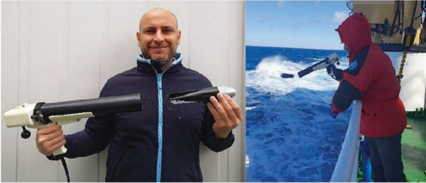
Fig. 3.4 Left panel: an XBT probe out of its canister and the hand launcher. Right panel: an XBT deployment by means of a hand launcher
