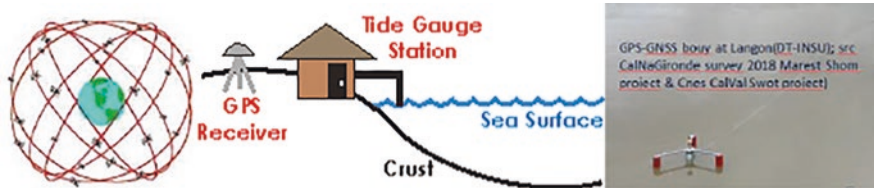
Fig. 10.9 (Left) Schematic view of GNSS constellation for precise positioning; (middle) gauge installation (src: PSMSL); (right) GPS-GNSS buoy (src: Insu) deployed during CalNaGironde-Marest survey, CNES Swot and Shom project [1]
