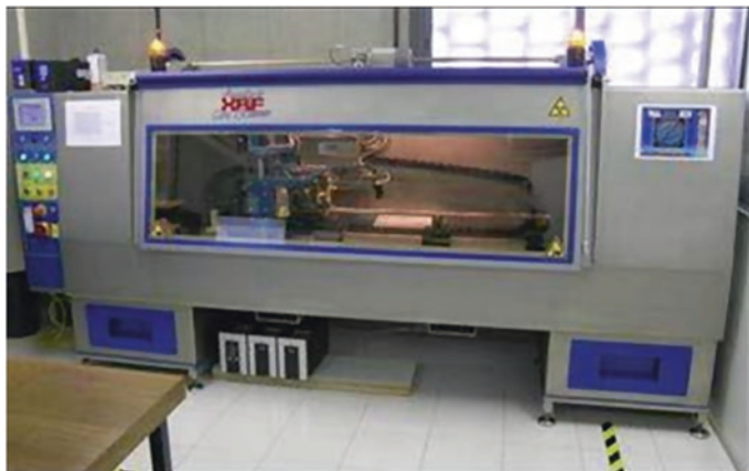
Fig. 11.11 The Avaatech XRF Scanner at the Laboratory of University of Barcelona (from Meo et al. [19])
