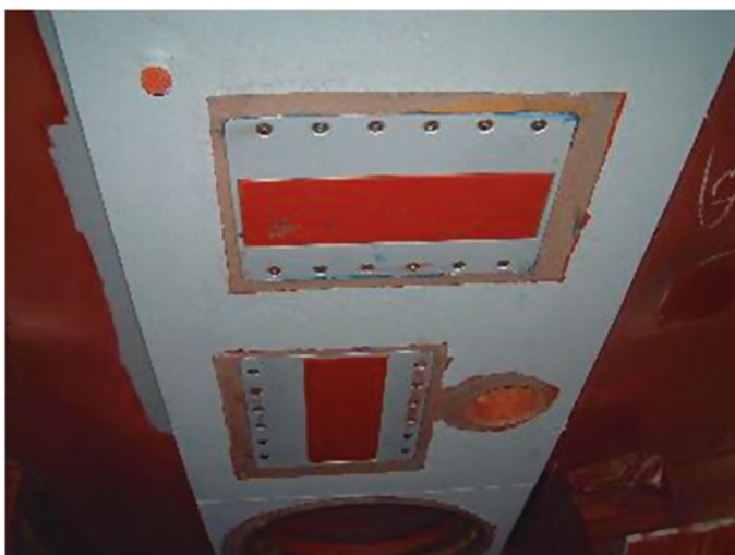
Fig. 1.2 Tx and Rx multibeam transducer (courtesy of Kongsberg Maritime AS)
