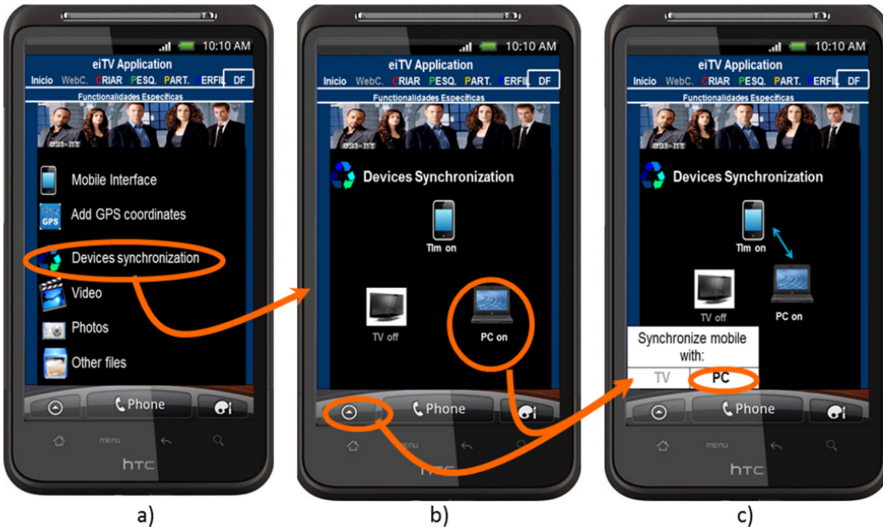
Fig. 4. eTV Devices Synchronization. Synchronizing devices: a) Options available at the DF functionality and ‘Devices Synchronization’ option being selected; b) Automatic detection on the connected interfaces. Viewer use the phone button in order to activate the menu to choose to which device synchronize his mobile; c) In this case is choosing PC (the only device on).
