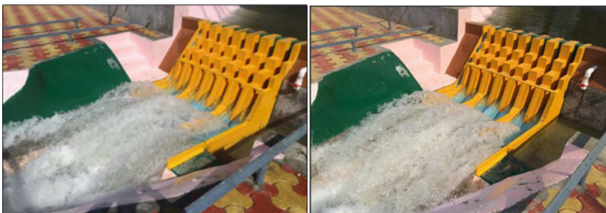
a) Ungated operation of spillway
