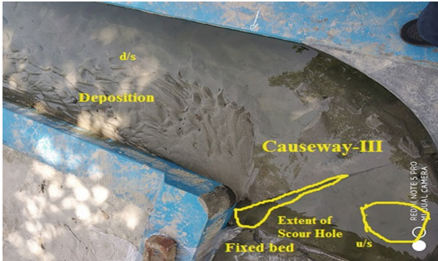
Fig. 32.10 Photogrammetric view of Scour around Causeway-III (Fixed Bed)
