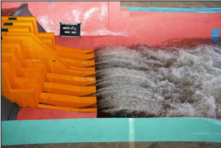
Photo 15.2 Performance of modified ski jump bucket (Discharge through the spillway, Q = 16,023 \text{ m}^3/\text{s} , at Full Reservoir Level (FRL))
