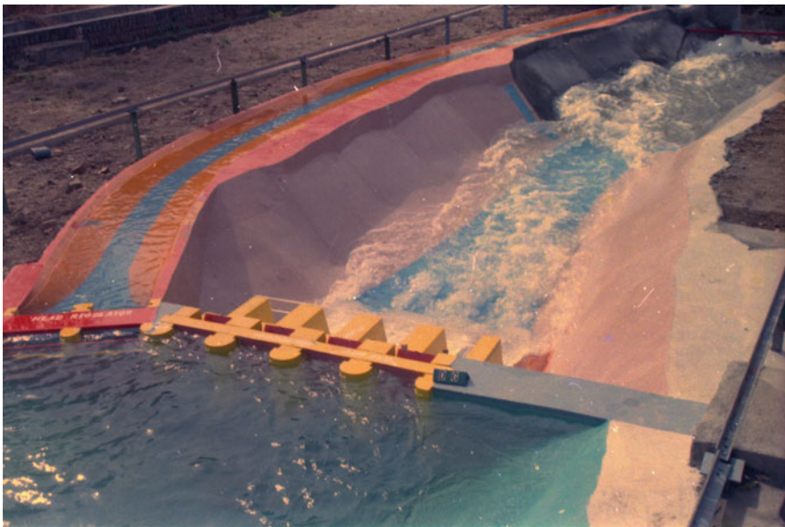
Photo 14.1 Flow conditions in open channel downstream of head regulator
