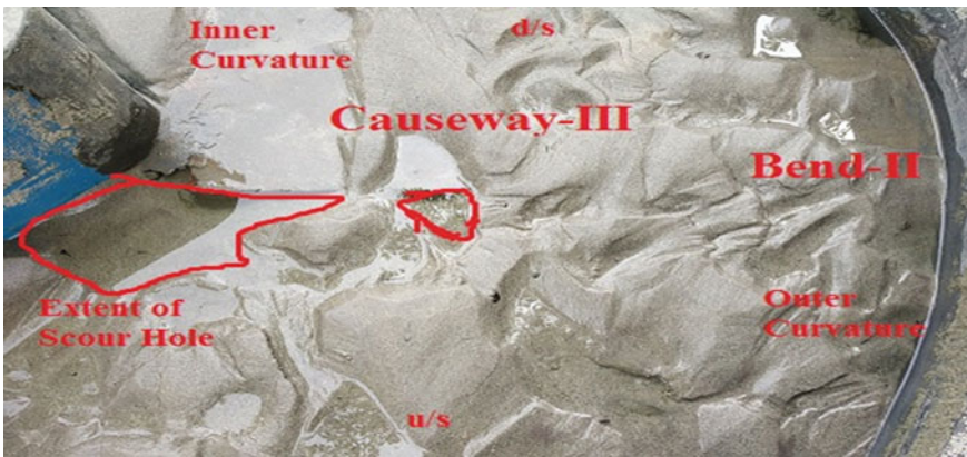
Fig. 32.9 Photogrammetric view of scour around causeway-III (Mobile Bed)
