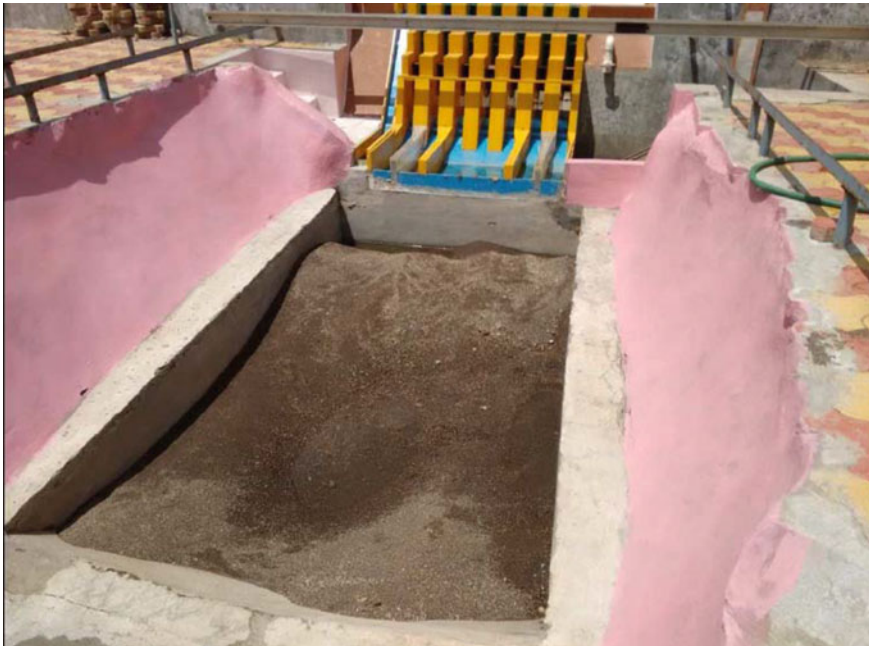
Fig. 28.12 Typical scour profile observed in the physical model
