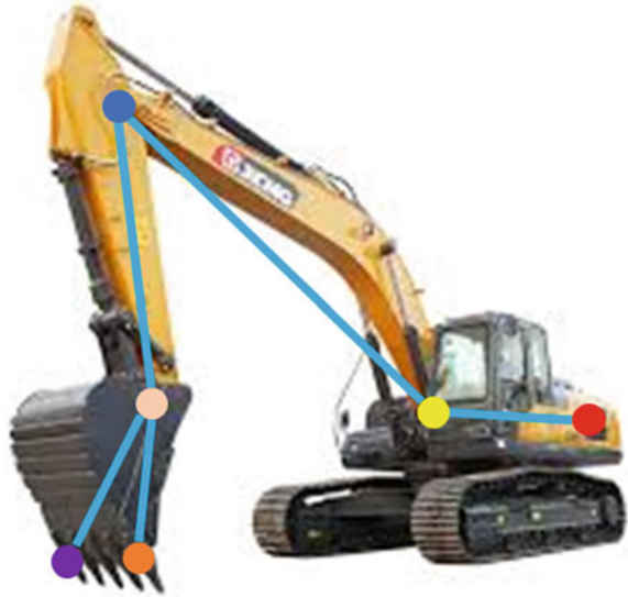
Fig. 12 Posture estimation of construction machinery
