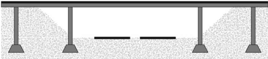
Fig. 5 Side view of a three-span highway beam bridge, where the main span goes over a road. For a more detailed view of the Z24 bridge, refer to [33]
