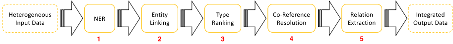
Fig. 1. The XI pipeline goes through a series of five steps to integrate semi-structured or unstructured content leveraging a knowledge graph
