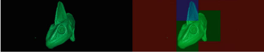
Fig. 11 The image on the right shows the used encoder settings for the image on the left. Tiles that are red used the LOW settings, i.e. the maximal compression, tiles that are blue use the MEDIUM encoder setting and the green tiles use the HIGH setting, i.e. minimal compression
