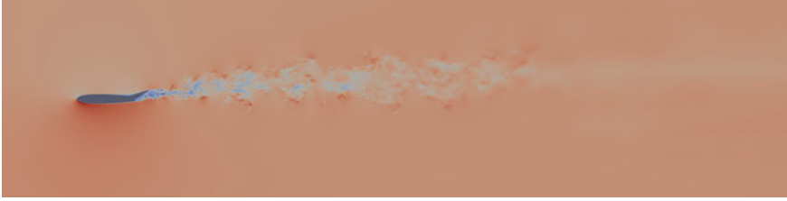
Fig. 8 From a 1M-way parallel PHASTA run on mi.ra at Argonne National Laboratory, this image is a zoomed-in view of a 2D slice from 3D volume. This numerical simulation models the flow over a vertical tail-rudder assembly for a geometry that exactly matches the configuration of an ongoing wind tunnel experiment. This image is reprinted from our previous work [1]
