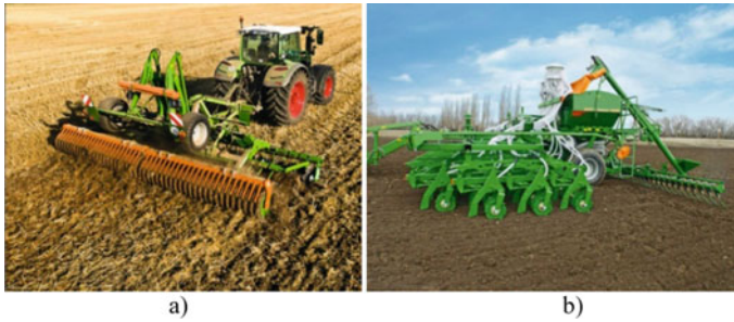
Fig. 1. a Catros disc harrow, b seeder Primera DMC (JSC “Eurotehnika” for moisture-saving technologies)
