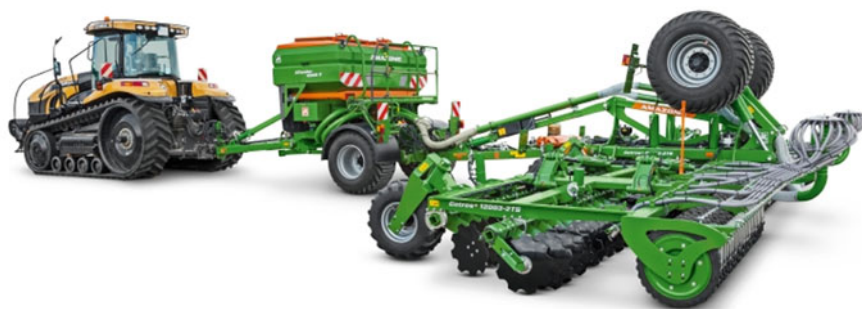
Fig. 6. An innovative soil cultivation and fertilizer complex in the trailed version X-TenderT with a Catros disc harrow
