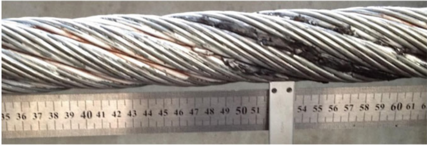
Fig. 5. Photo of a defective section of a rope with a diameter of 48 mm, construction 6 \times 26 (1 + 5 + 5/5 + 10) WS-SPC 1600 B zZ with “waviness” defect.
