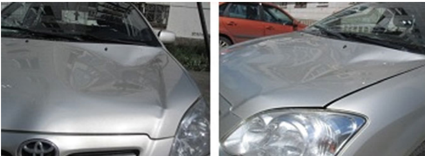
Fig. 7. Photos of a car damaged by falling snow mass
