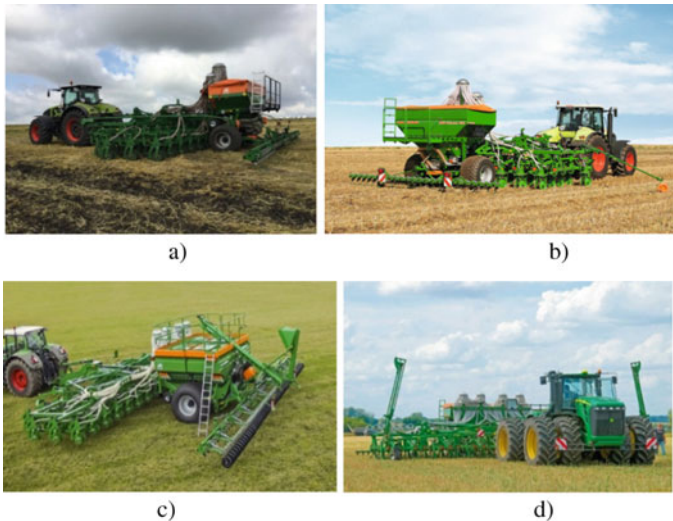
Fig. 1. DMC seeders of various working widths (m): a 3.0; b 6.0; c 9.0 d 12.0
