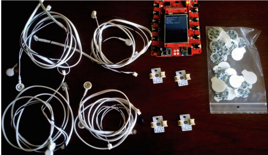
Fig. 2 MySignals platforms and sensors used for acquisition of EMG signals
