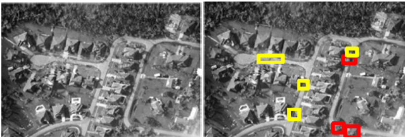
Fig. 7. Example of an obtained city image and identification of blockages or suspicion of blockages
