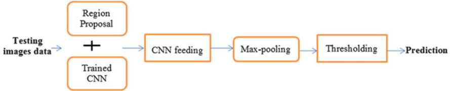
Fig. 26.7 Logo recognition testing process (Source: Authors' aggregation)
