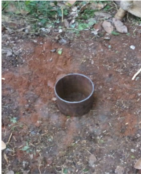
Fig. 15.2 Infiltrometer installed at the Study Area-2
