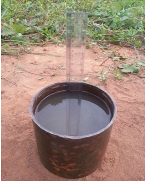
Fig. 15.1 Infiltrometer installed at the Study Area-1
