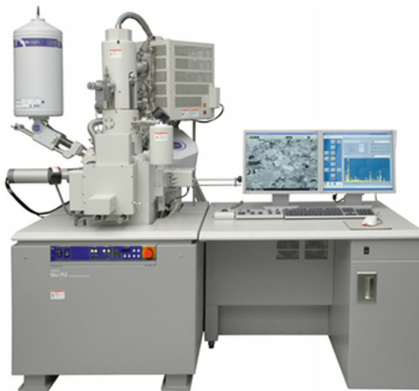
Fig. 5. Hitachi SU-70 network scanning microscope [5]
