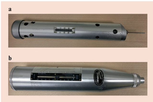
Fig. 9.56 Testing devices for the hardness of materials with dynamic methods ((a) Pilodyn and (b) Schmidt–Hammer, Proceq, Zurich, Switzerland). (Photo P. Niemz)
