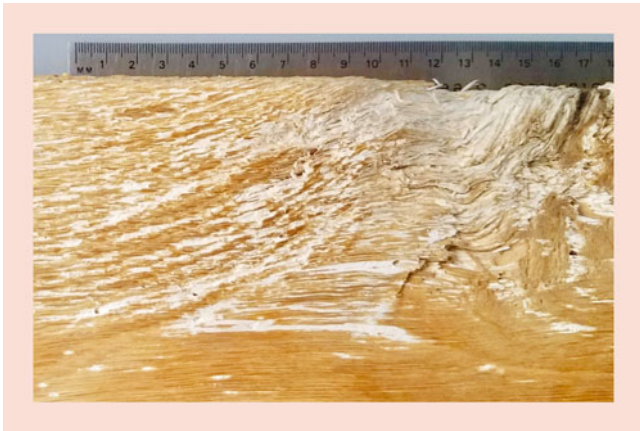
Fig. 4.4 The classic stringy and bleached appearance of white rotted wood in a hardwood. This type of decay is often colloquially referred to as spongy white rot, or stringy white rot
