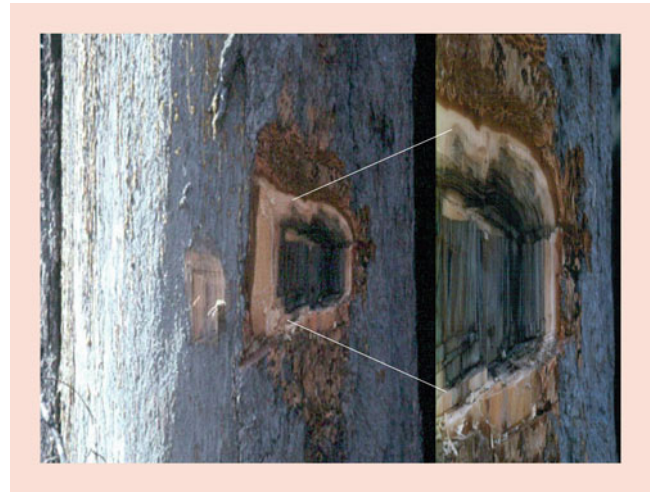
Fig. 4.9 “Mount St. Helen’s blue stained wood.” This purple to black stain developed in the interior sapwood of dead and dying Douglas fir trees on the slopes of Mount St. Helens after it erupted in the 1980s. Although it was considered to be a fungal blue stain by local mills, analysis showed that high levels of iron present in the dark zones were responsible for the discoloration
