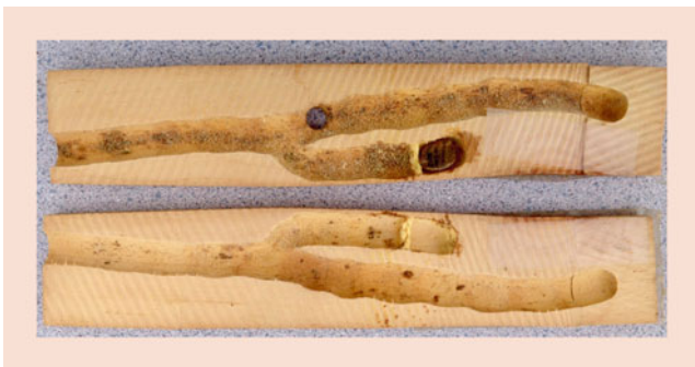
Fig. 4.18 Carpenter bee damage to wood that was exposed by sawing longitudinally through the nest chamber. (Note “bee bread” pellet of pollen and nectar at the end of the branching gallery section, and entrance hole in the center of the upper section)
