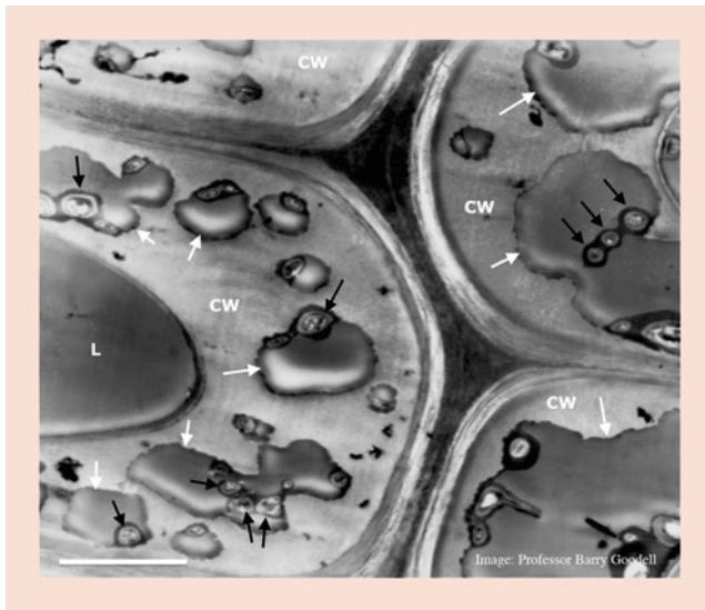
Fig. 4.7 Transmission electron micrograph of a southern pine wood cross-section. The wood was used as a cooling tower slat and was being decayed in a Type I soft rot attack. The image shows portions of four pine tracheids with fungal hyphae decaying parts of the each of the cell walls (CW) of the tracheids. Cavity formation shows the fungal hyphae growing within the S2 layer of the wood cell walls and producing cavities (white arrows) surrounding individual hyphae (select hyphae are identified with black arrows). The cavities often coalesce in this heavily degraded sample
