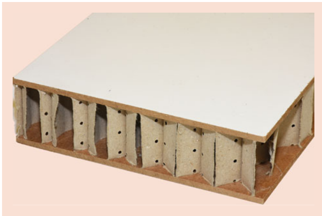
Fig. 35.39 Sandwich element with kraft paper honeycomb structure. (Photo D. Sandberg)
