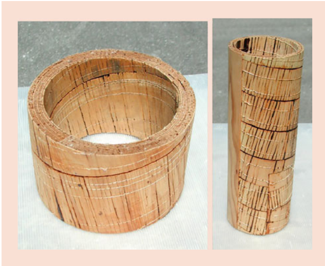
Fig. 35.59 Segments of cylindrical LVL
