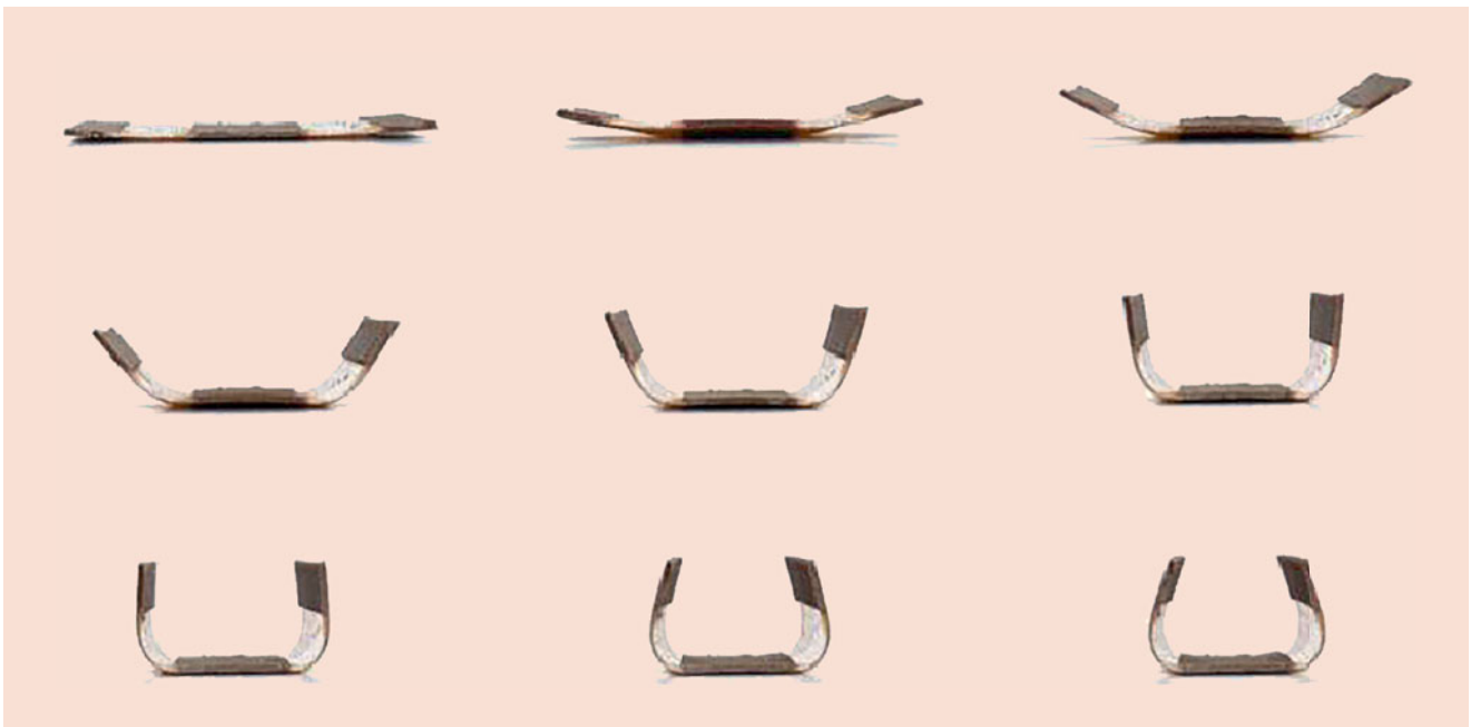
Fig. 35.17 A series of photographs showing a multimaterial printed wood composite developed by the Self-Assembly Lab at Massachusetts Institute of Technology (MIT), that self-transforms from a flat sheet into a symmetrically folded structure [162]
