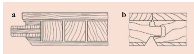
Fig. 35.48 Typical parquet system with tongue and groove. The geometry with gaps between adjacent middle and bottom layers allows a tight alignment of the top layer: (a) front end connection with glued-in plywood strip, and (b) length-side connection
