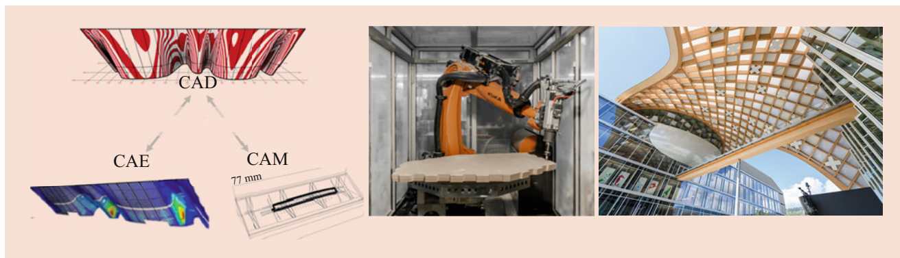
Fig. 35.52 Digital planning process CAD-CAE-CAM interfaces in the construction of the Swatch headquarters, Swatch and Omega campus in Biel, Switzerland. New dimensions in complexity in timber construction. (Shigeru Ban Architects, photo Blumer-Lehmann AG, Switzerland)
