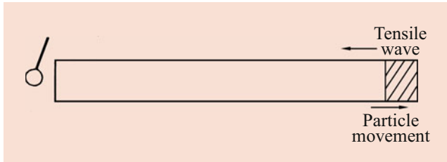
Fig. 19.8 Travel of compression wave along bar. The forward-moving wave impinges on the free end of the bar, is reflected back as a tensile wave, and begins to travel back down the bar
