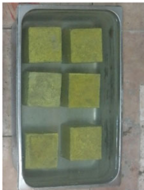
Fig. 2 Results of water absorption measurements
