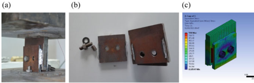
Fig. 5 Photo of the test sample of the C345Comb group: a , b photo of the sample after the tests; c the result of numerical simulation of the sample of the third group
