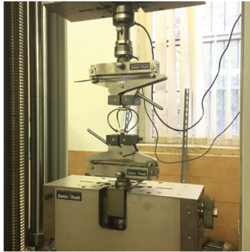
Fig. 2 The wire rope-based device subject to the experimental testing campaign
