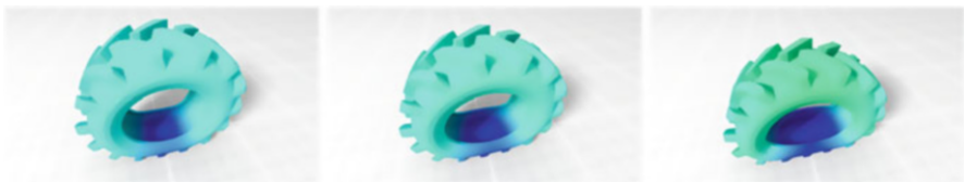
Fig. 2 Test 5. Large deformation of a finite element mesh colliding with a plane. Thanks to the non-smooth formulation, large time steps can be used (only ten steps have been used from start to end), and no penalty parameters must be used in contact points. Contacts between lugs and ground show zero interpenetration regardless of the stiffness of the mesh
