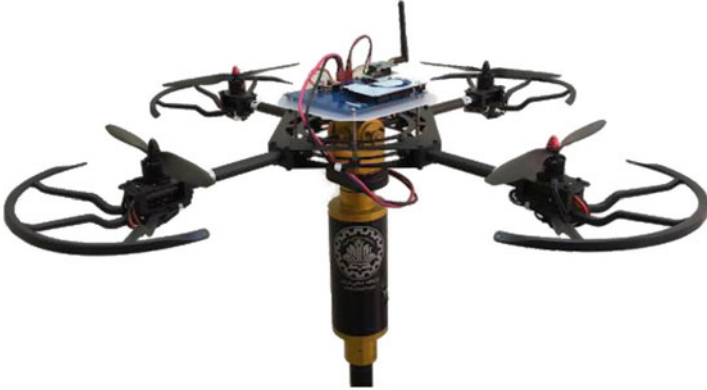
Fig. 2 The captive test stand
