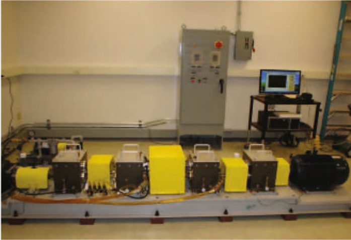
Fig. 1 Gear-train experimental setup, four gray metal boxes denote 4 gearboxes
