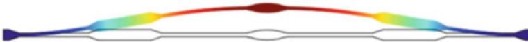
Fig. 3 The fundamental flexural mode of the new design for maximizing the hardening behavior of a clamped–clamped beam. The color denotes the total displacement. The mode shape is obtained by using COMSOL Multiphysics 5.4 with 2D solid element
