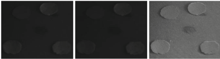
Fig. 50.7 530 nm radiation: parallel axes (left), orthogonal axes (middle), processed image (right)
