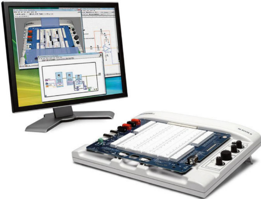
Fig. 8.1 Computer-based virtual instrumentation workstation using NI ELVIS II platform
