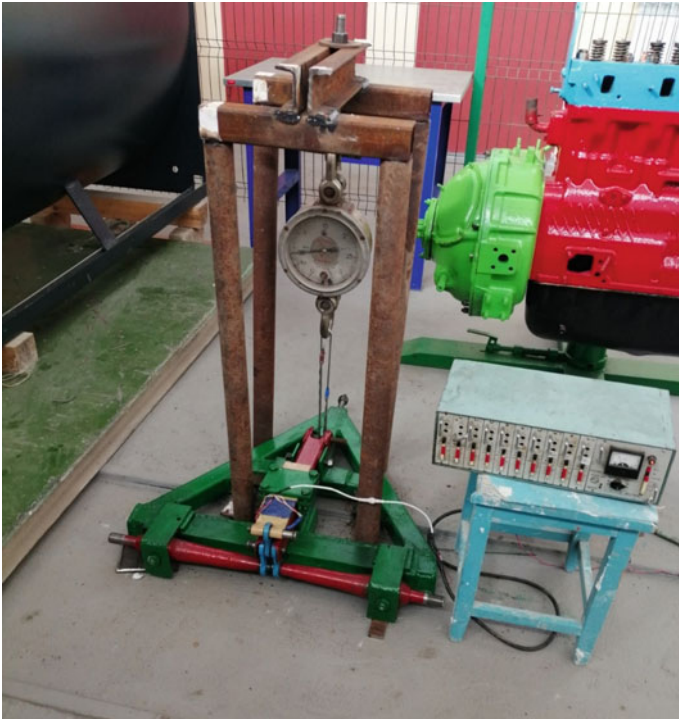
Fig. 6 Experimental determination of the characteristics of the proposed device on a load stand
