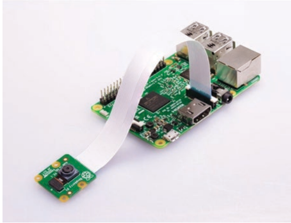
Fig. 8.2 Raspberry Pi with camera module [17]
