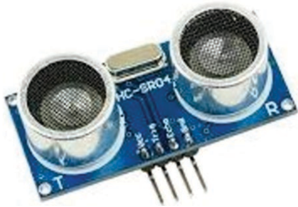
Fig. 8.3 Ultrasonic range sensor (Hc-Sr04) [18]
