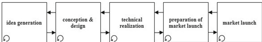
Fig. 2. Proposed process model for the development of smart service in supplying companies
