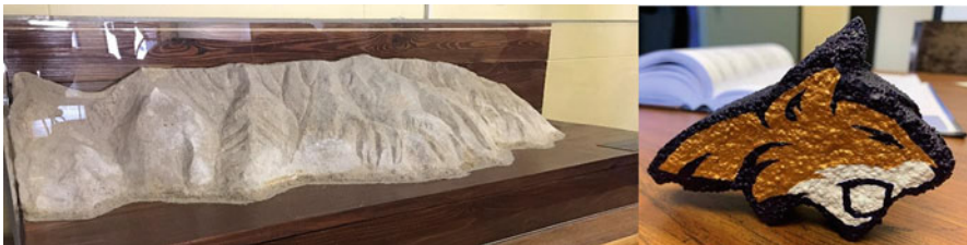
Fig. 12 (Left) 0.9\text{ m} \times 0.3\text{ m} \times 0.3\text{ m} biomineralized replica of the Bridger Mountain range. (Right) Biomineralized replica of the Montana State University mascot, the Bobcat
