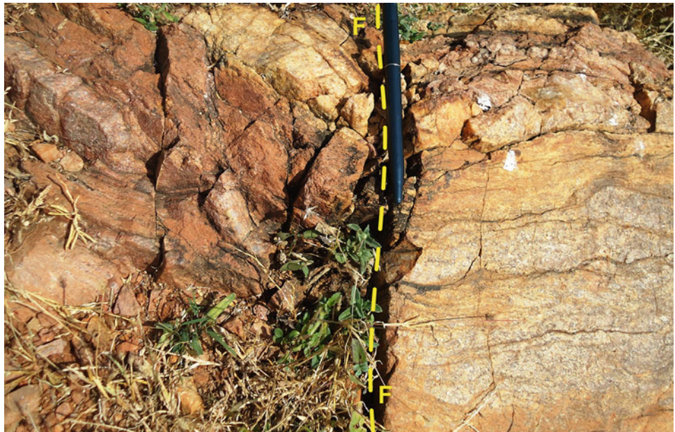
Fig. 9.50 Abrupt change in dip of strata due to the presence of a fault (yellow dashes) in quartzitic rocks of Bundelkhand craton, central India. The dip of the strata, in both amount and direction, is different on either side of the fault. (Photograph by the author)
