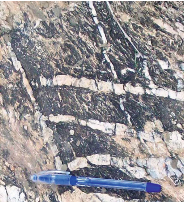
Fig. 13.12 Filled joints. Joints if filled with secondary minerals are called veins. In the photograph, gneissic rocks show two sets of joints at high angles. Due to filling of secondary silica, these joints can be called silica veins. (Photograph by the author)
