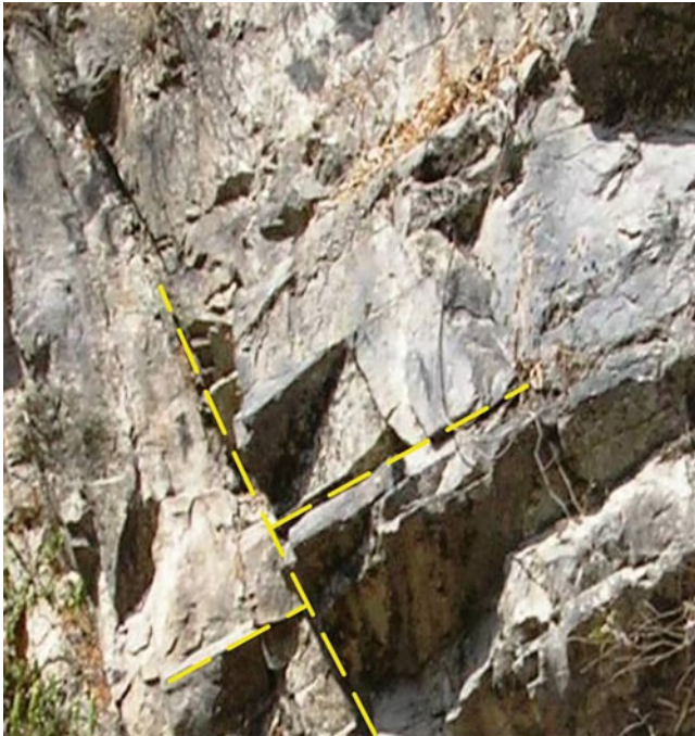
Fig. 13.2 Shear fractures in massive limestone occurring as planes of discontinuity that is associated with small shear displacement (shown by yellow dashes)
