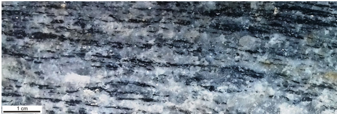
Fig. 14.2 Photograph of a gneiss showing foliation in hand specimen with two distinct domains. The cleavage domain is shown by dark-coloured bands given by biotite, while the intervening space represents the microlithon domain. (Sample courtesy Geology Museum, University of Lucknow)
