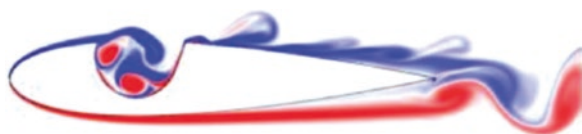
Fig. 2.9 The flow over an airfoil with a cavity on its suction surface (Olsman and Colonius 2011)
